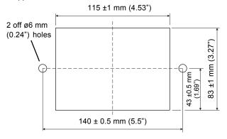
The panel should be pieced with a square cutout for the display, and drilled with two 6 mm (0.24") holes for the screws. The main unit is offered up to the square cutout with the display
